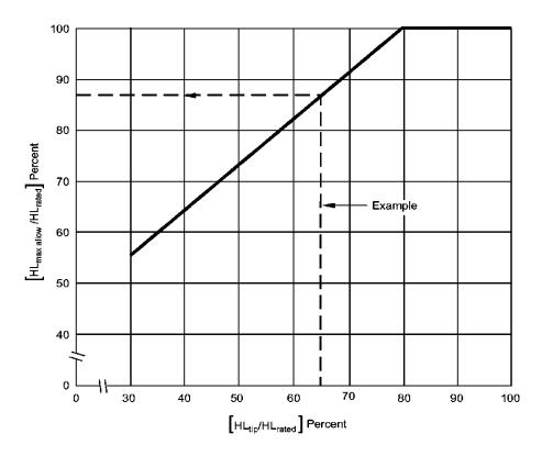
Some portable masts with guylines may have maximum rated hook load capacities (HL<sub>rated</sub>) that, if applied, could result in overloading of guyline anchors. In such cases, it is necessary to determine the maximum allowed hook load (HL<sub>max allow</sub>) which will prevent anchor overload. The chart above can be used to determine the magnitude of mast derating required to insure that anchor capacities shown in Figure 3 are not exceeded.
