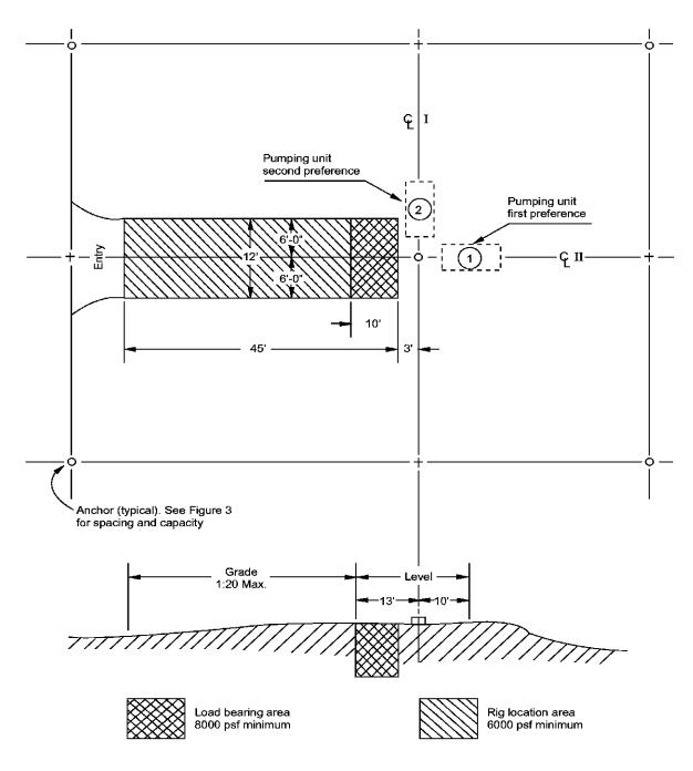
Load bearing area: Compacted sand or gravel requiring picking for removal or better base. Safe bearing capacity desired—min., 8000 psf, level and drained.
